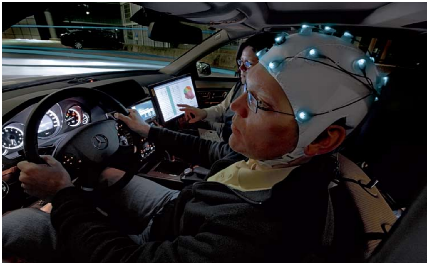
A significant aspect of the "Vision of Accident-free Driving" is maintaining driver fitness. In the Mind-Lab mobile research laboratory, scientists at Daimler are investigating cognitive subconscious driver behavior on the basis of neurophysiological measurements, in order to further improve assistance systems.
